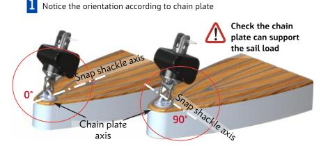
Assemble the snap shackle to the drive unit (2 possible positions)
