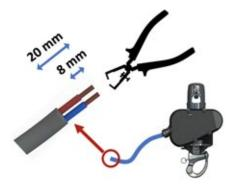
**Weld** with tin the wire to the mobile plug
