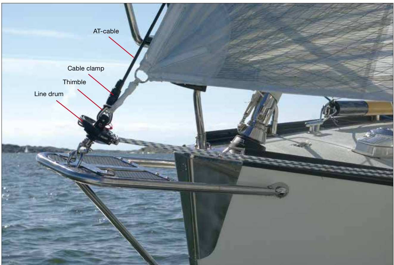
A Seldén CX15 Code 0 furler and a Race80 Bowsprit from Båtsystem, Sweden. www.batsystem.se . The luff load on a Code 0 is more than the double compared to an asymmetric spinnaker. Therefore, a sturdy bowsprit is required.
