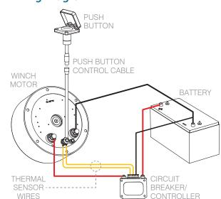
Motor units are supplied with installation manual, push button, 1000mm (39<sup>+</sup>) push button control cable, circuit breaker/controller and terminal extensions. A secondary push button RA866000, RA866010 or RA866020 can be added to the installation <u>only</u> if specified with the original order, and may not be retrofit.
