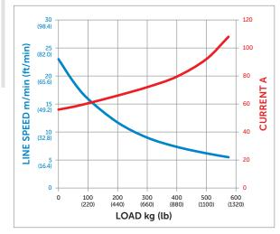
The motor will cut-out at pre-determined current and temperature limits.
