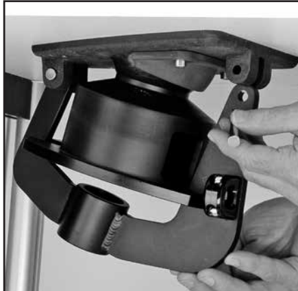
Remove Bridge Assembly
