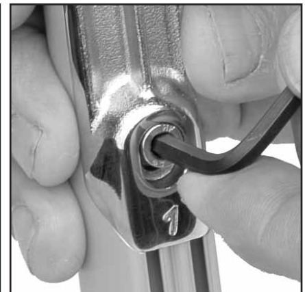
Slide screw up and hold.
