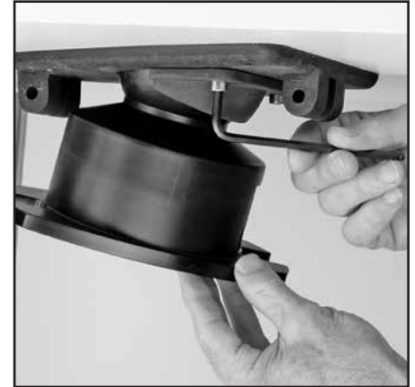
Remove Ball/Spool Assembly
