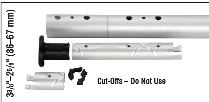
3 3/8"–2 5/8" (86–67 mm) Do not use plastic bushing above top connector. Cut connector right at cross formed by glue dispersion channels. Use single foil screw in top foil only.
