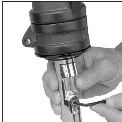
Loosen screw one revolution only .
