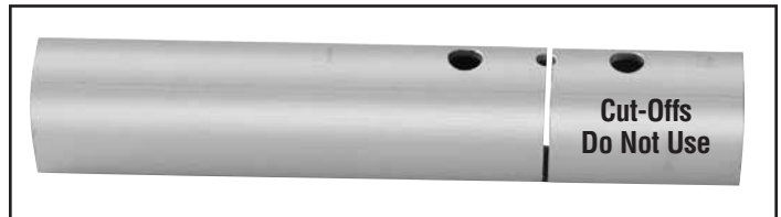
*To allow for saw cut, position blade so upper half of middle hole is preserved.
