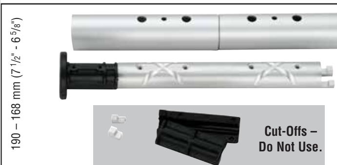
190 – 168 mm (7 1/2" – 6 5/8") Do not use plastic bushing above top connector. Shorten top of connector and if necessary shorten trim cap.
