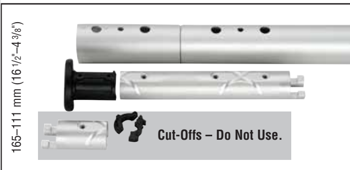
165 – 111 mm (6 1/2" – 4 3/8") Do not use plastic bushing above top connector. Cut connector right at cross formed by glue dispersion channels. Use single foil screw in top foil only.
