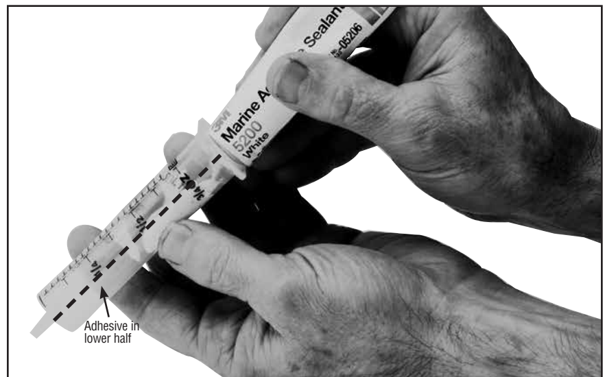
Loading Injector with Adhesive
