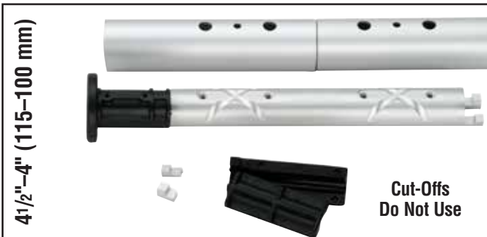
4 1/2"–4" (115–102 mm) Do not use plastic bushing above top connector. Shorten top of connector and if necessary shorten trim cap.
