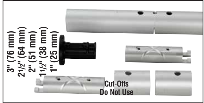
3"–1" (76–25 mm) Shorten top foil and adjoining full length foil so two screws are used to assemble joint instead of four. Do not use plastic bushings above top connector.
