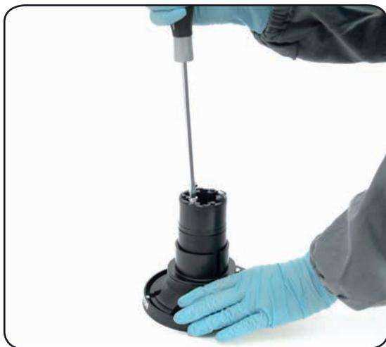
6. Completely unscrew the three screws n°16
