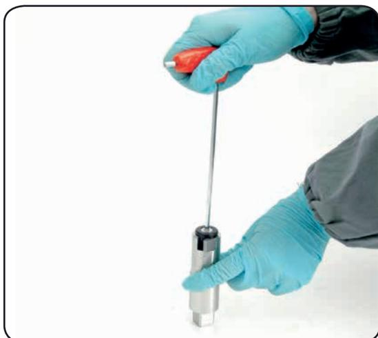
Unscrew the screw n°10 and remove
