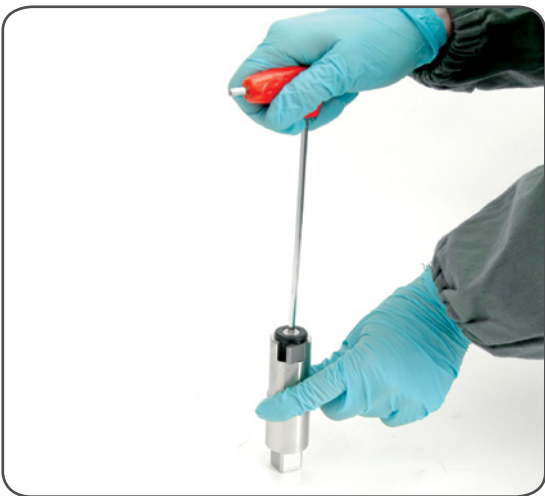
9. Unscrew the screw n°10 and remove the washer n°9 (⚙️4Nm/35 in-lb)
