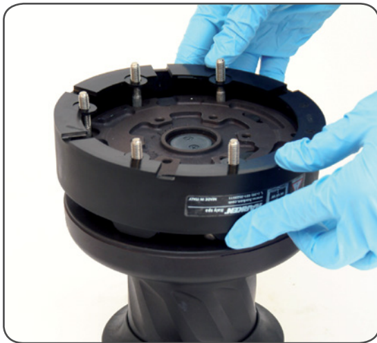
4. Reposition the skirt n°2 in its housing
