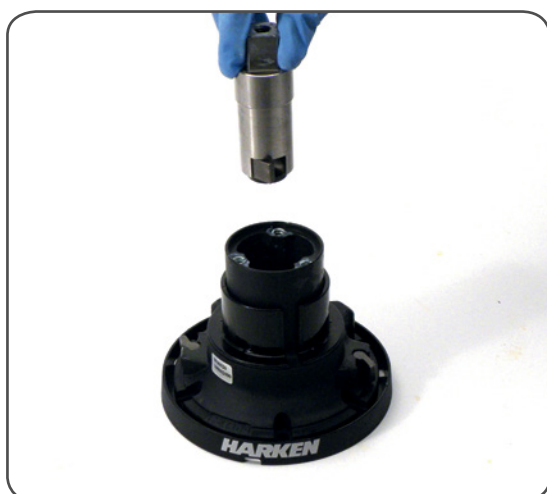
5. Slide out the central shaft n°7 and the bushing of the assy housing
