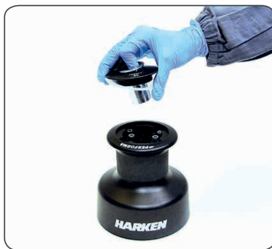
2. Slide off the hub n°28 and the cover n°25 and the washer n°30
