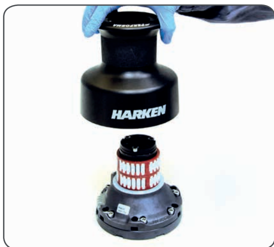
3. Lift off the drum n°22
