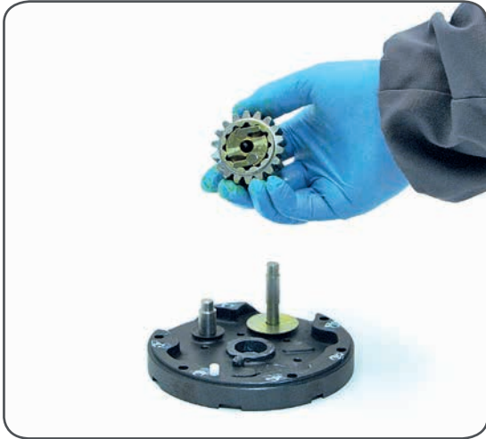
14. Remove the pawls n°5. To facilitate the operation press the spring against the pawl with a blade.
