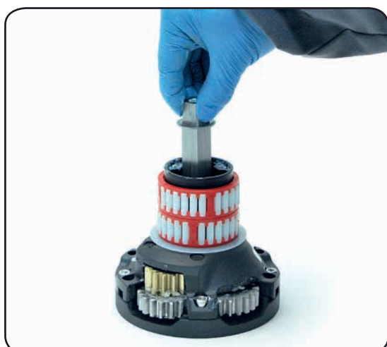
6. Slide out the central shaft n° 19
