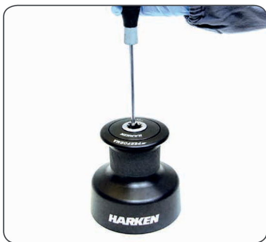
1. Unscrew the central screw (⚙️ 2Nm/18 in-lb)
