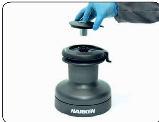
2. Slide off the assy socket n°28 and the cover n°27
