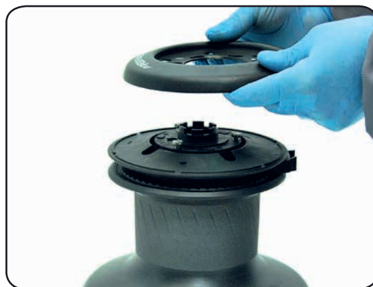
4. Remove the stripper arm n°25 by rotating and lifting it.
