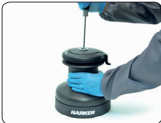
1. Unscrew the central screw ( \approx 2\text{Nm}/18\text{ in-lb} )
