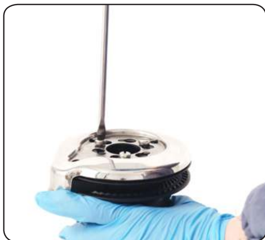
3. Unscrew the three screws n°28 ( \approx 4\text{Nm}/35\text{ in-lb} )
