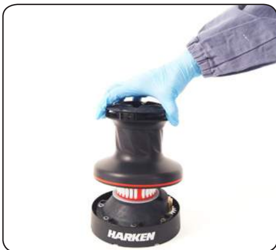
5. Lift off the drum n°23
