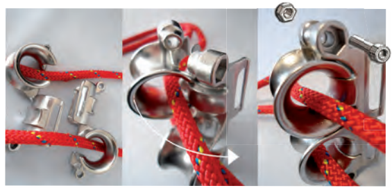
Open the twin fairlead to introduce the existing spliced furling line through the ring.
