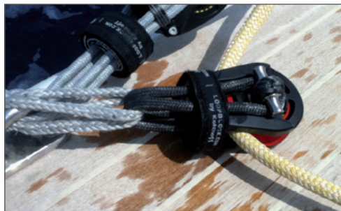
LOOP® Block 60NB as a Code Zero Block on a SWAN 60.
