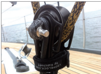
LOOP® Block LB-60-4BB on a Hanse 630 Race.
