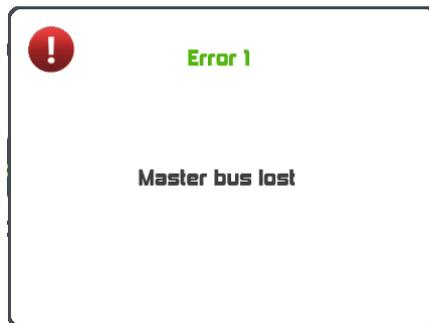
The “master” display is unplugged or out of order. This can be solved by replacing the “master” display by another one. (Refer to “Toplines addresses” section).
