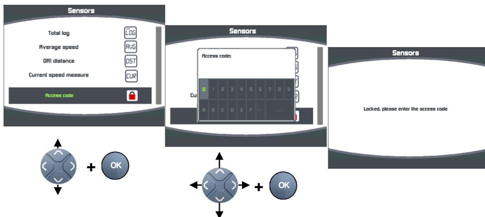
Procedure to unlock the sensor menu:
