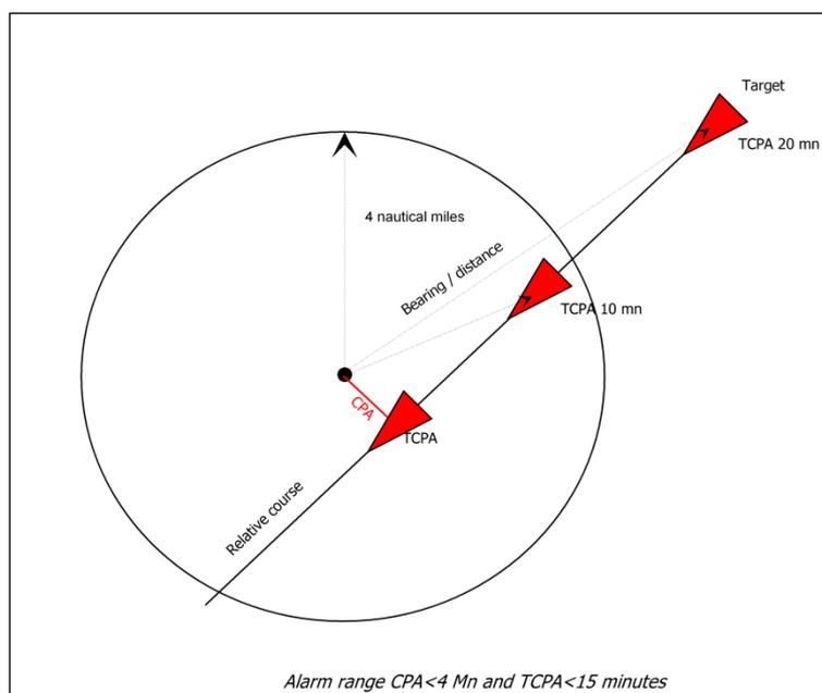
The alarm has been set for « **CPA < 4 Mn and TCPA < 20 minutes** ». As a result, **CPA** being below 4 miles and the **TCPA** calculated value being below 20 minutes, the **Multigraphic** triggers an alert.
