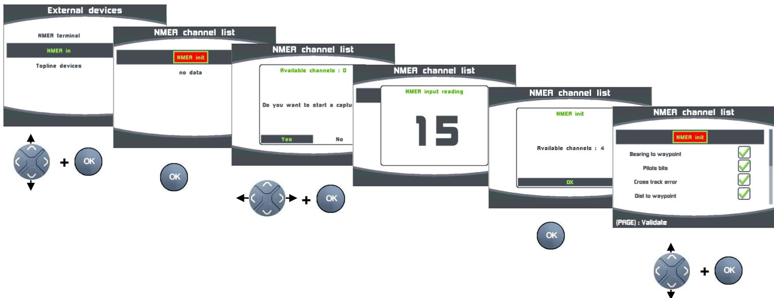
All NMEA channels are activated by default. You can choose to inhibit some channels. This is done by selecting the chosen channel and pressing
