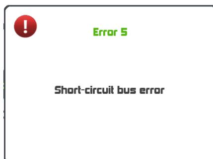
The black wire of the Topline bus cable, carrying the data is in short-circuit with one of the 2 other wires. This can happen in a junction box, the cable itself or one of the units connected to the bus.
