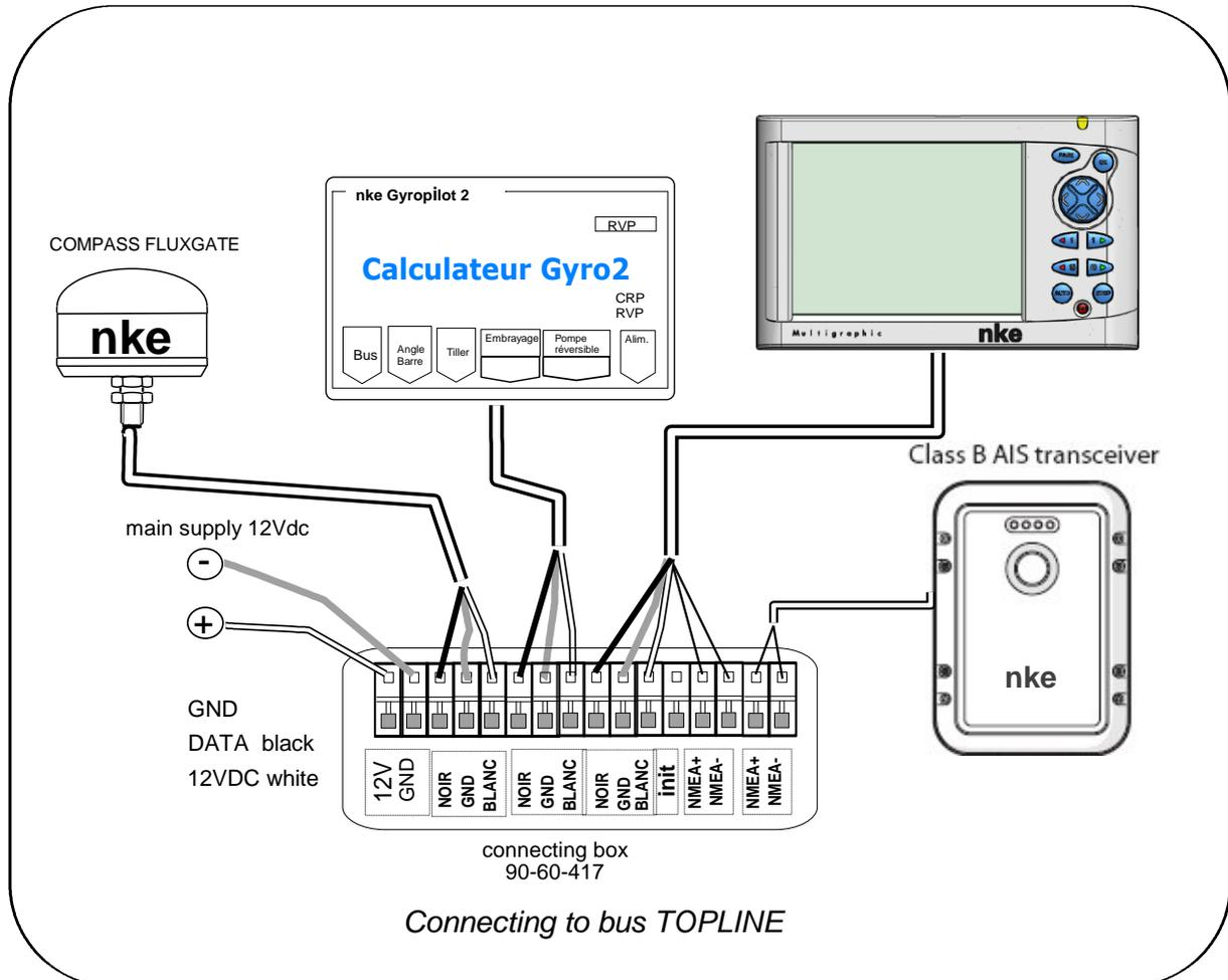
Should you want to cut the bus cable to length, uncover and tin the wires before connecting them.
