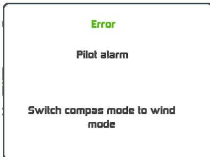
When the pilot in compass mode and an alarm has been set this will be displayed when the compass heading is over the defined range. Press any key to inhibit the alarm for 7 minutes.
