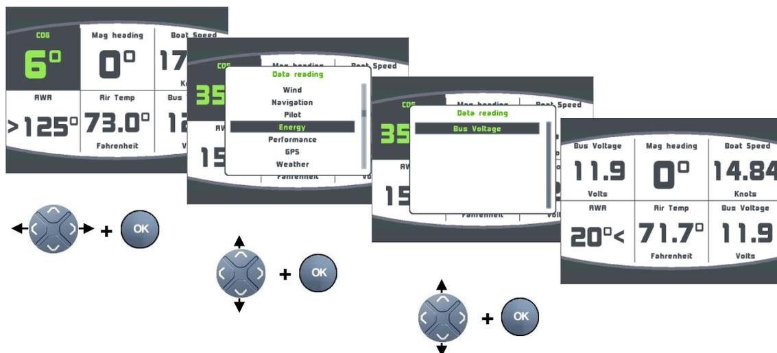
This modification has not been saved and the previous layout will return the next time the system is powered on.
