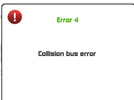
2 similar sensors are connected to the bus and transmit the same data, or an NMEA input has been set for the same data as a sensor present in the bus. Check the connected sensors and reset the NMEA inputs.
