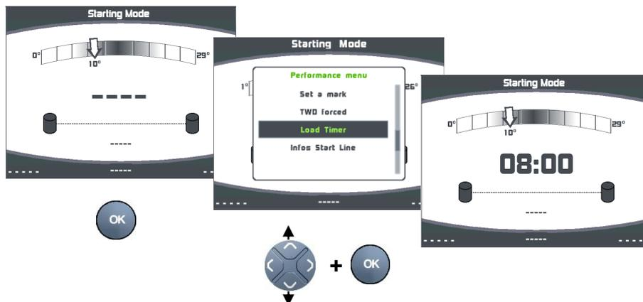
A press on “OK” starts the count-down. A second press on “OK” resets the timer on T2.
