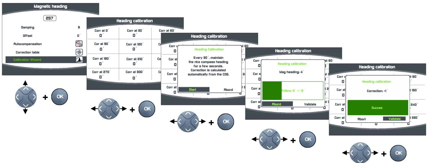
Press “**OK**” to save the new correction. You can highlight “Abort” and press “OK” if you want to cancel a correction. Repeat this operation every 30° to fill the whole correction table. The compass will have its deviation curve implemented once this table is completed.
