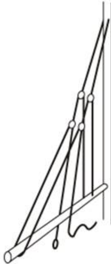
Diagram C - Reeving the Lazy Jack around the boom.
