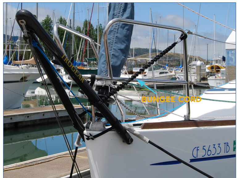
Fig 14: Showing Bungee Cord and Stop Strap.
