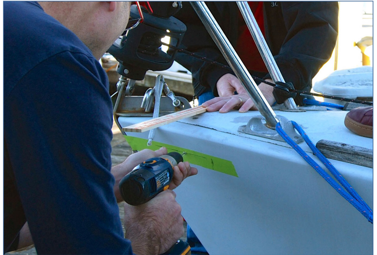
Fig 6: Drill a pilot hole first.
