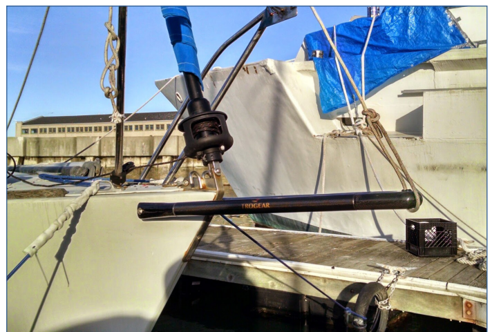
Fig 12: Temporarily secure the Bowsprit with a line
