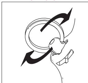
Lift and rotate pull-pin ninety degrees
