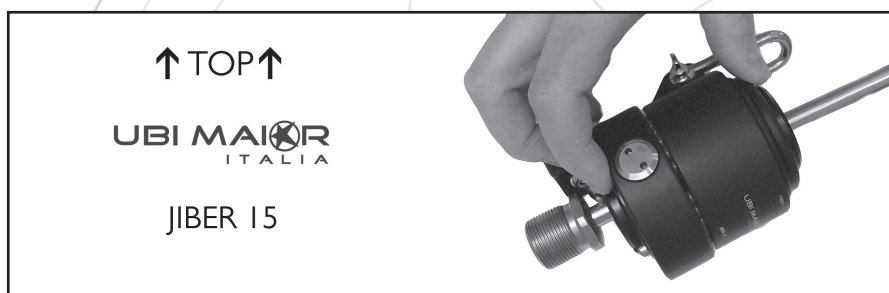
INSERT THE SHUTTLE INTO THE ROD IN THE CORRECT DIRECTION (AS SHOWN)
