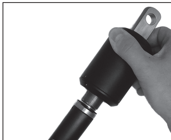
SCREW THE SWIVEL ONTO THE CONNECTOR (ANTI-CLOCKWISE) UNTIL IT IS FULLY SCREWED ON
