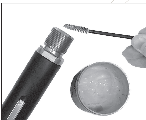
APPLY TEF-GEL® TO THE INSET HEAD OF THE ROD TERMINAL
