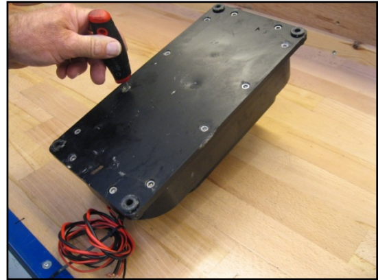
Dismount 12pcs M6 allen screws from the bottom of the drive
