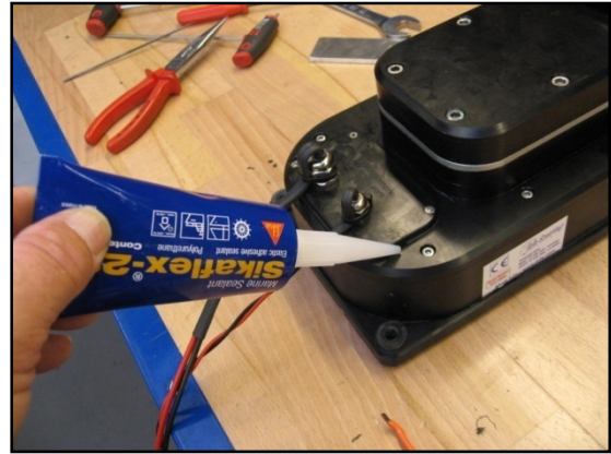
Use sikaflex around cover for wiring
