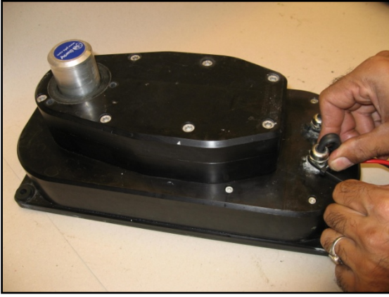
Use strips around the cable and cable screws so that it looks as on the picture
