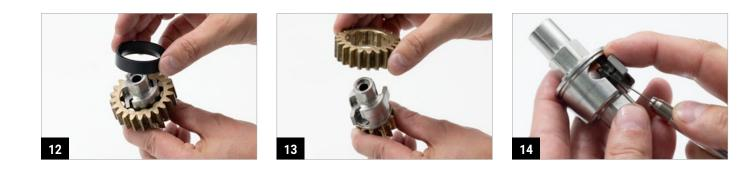
15. Clean all gears, pawls and pawl springs with a brush and white mineral spirits to remove old grease and contaminants. Reassemble gear assemblies.
