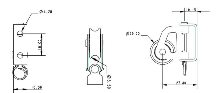
Details: A 20mm ball bearing sheave riveted to a stainless steel frame which can move through 180 degrees. The body is fixed to the backing plate with a removable clevis pin for easy removal and installation.
