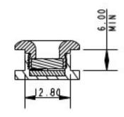
Details: We have continued with the development of our range of deck bushes with this range of through deck pad eyes that incorporate a Tii attachment.
